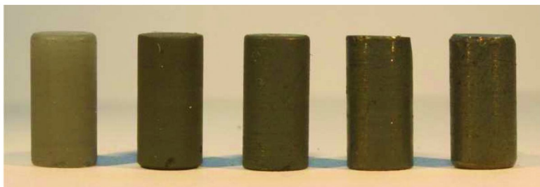
Figure 4. Picture displaying the extruded AIFA composites that have been machined into 4 mm diameter x 8 mm length cylinders with (left to right) 0, 10, 30, 50 and 60 wt% aluminum nanoparticle content in a poly(PFDMA) matrix.
