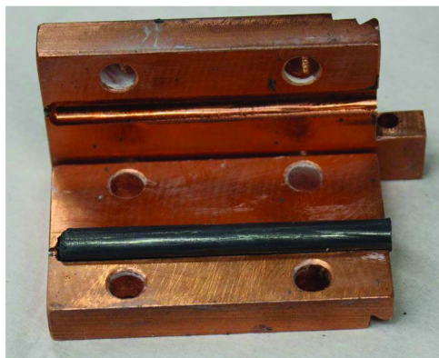
Figure 3. Image displaying a clamshell mold with an extruded aluminum nanoparticle/fluorinated polymethacrylate composite.
